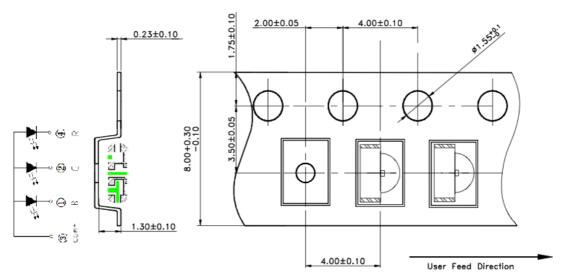
Unit: mm Tolerance: +/-0.10 mm
