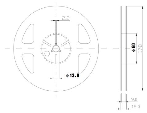
Unit: mm Tolerance: +/-0.15mm
