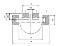
Figure 1. IN-S126TASRGB Solder Pattern
